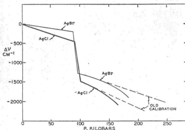
FIG. 1. Absorption edge versus pressure, AgCl and AgBr.
