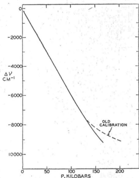
FIG. 2. Absorption edge of sulfur versus pressure.
